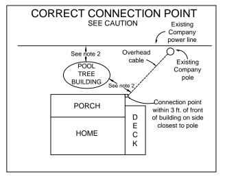
The Company will not install an electrical facility over a pool, building, shed, or deck.
