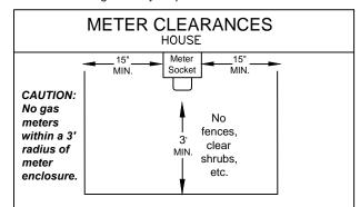
For residential service, the meter is to be located on the outside of the building on the side of the residence within three feet of the front wall and outside of the fences on the side most economical to reach the company's facilities. Main Breaker should be located outside within 2 feet of meter.
